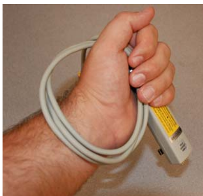
Figure 6 Recommended Coil for Storage
