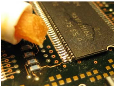
Figure 57 Fluxing of the Target Points
