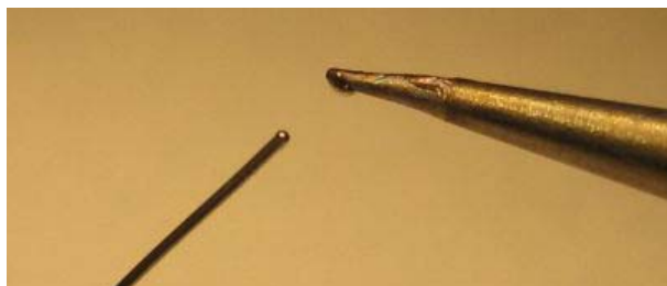
Figure 58 Small Amount of Solder Added to Soldering Iron Tip
