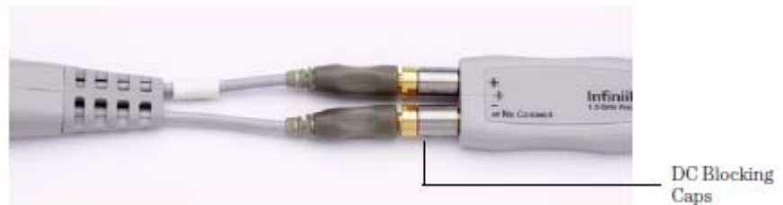
Figure 16 Blocking Caps Between Probe Amplifier and Head
