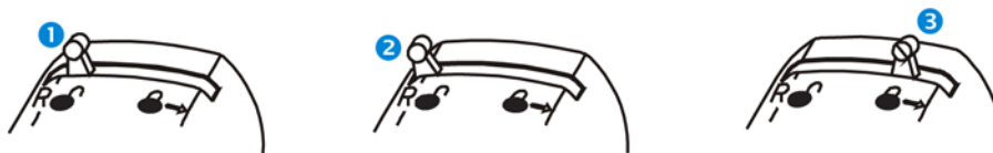
Figure 7 Properly Connecting a Probe to the Oscilloscope
