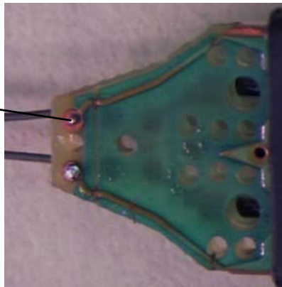
Figure 83 Wire Cut Flush with Solder pad
