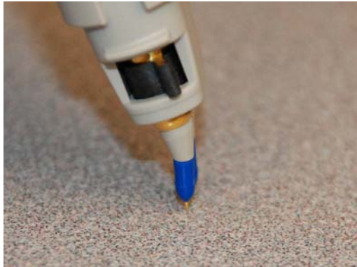
Figure 47 Proper Vertical Orientation of the Blue Tips
