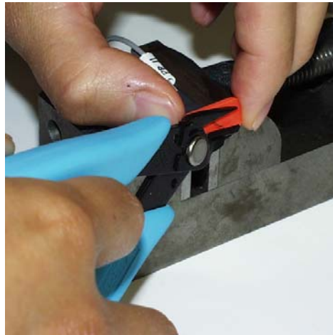
Figure 85 Cutting Wires Flush with Gauge
