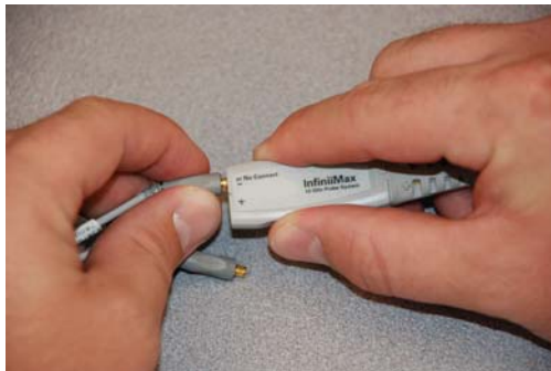
Figure 4 Properly Pulling the Probe Head Straight Out
